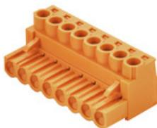
Female plug with clamping-yoke screw system for connecting wires with straight (180°) outlet direction. The female connectors provide space for labelling and can be coded. Fastened by means of a flange or release latch. They also provide an integrated plus/minus screw, protection against faulty insertion of the wire, and they are delivered with open clamping yokes. HC = High Current.
