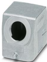
Sleeve housing B6, for single locking latch, material: Die-cast aluminum, salt water resistant, cable outlets: 1, lateral, 1x Pg13,5, height: 52 mm, cable gland: none, Standard
