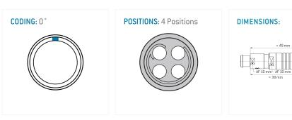
The pin layout corresponds to the view on the termination area
