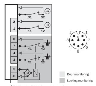
$\ensuremath{\mbox{\fontfamily}}$  Positive action N/C locking monitoring contact
