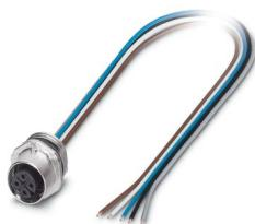
Device connector front mounting, Universal, 5-position, Socket, straight, M12-SPEEDCON, coding: A, on free cable end, Front mounting, M16 x 1.5, Individual wires, cable length: 2 m, 0.34 mm<sup>2</sup>, TPE litz wire
