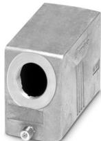
Sleeve housing B16, for single locking latch, material: Die-cast aluminum, salt water resistant, cable outlets: 1, lateral, 1x M32, height: 60 mm, cable gland: none, Standard
