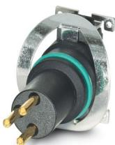
Contact carrier, 3-position, Pin, straight, M8, coding: A, PCB mounting, SMD reflow, Alternative product in accordance with RoHS II without Exemption 6c (Pb < 0.1 %) item no.: 1308281
