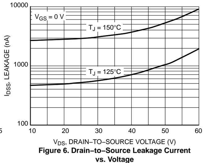
Figure 6. Drain-to-Source Leakage Current vs. Voltage
