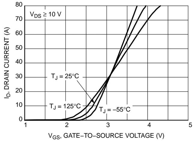
Figure 2. Transfer Characteristics
