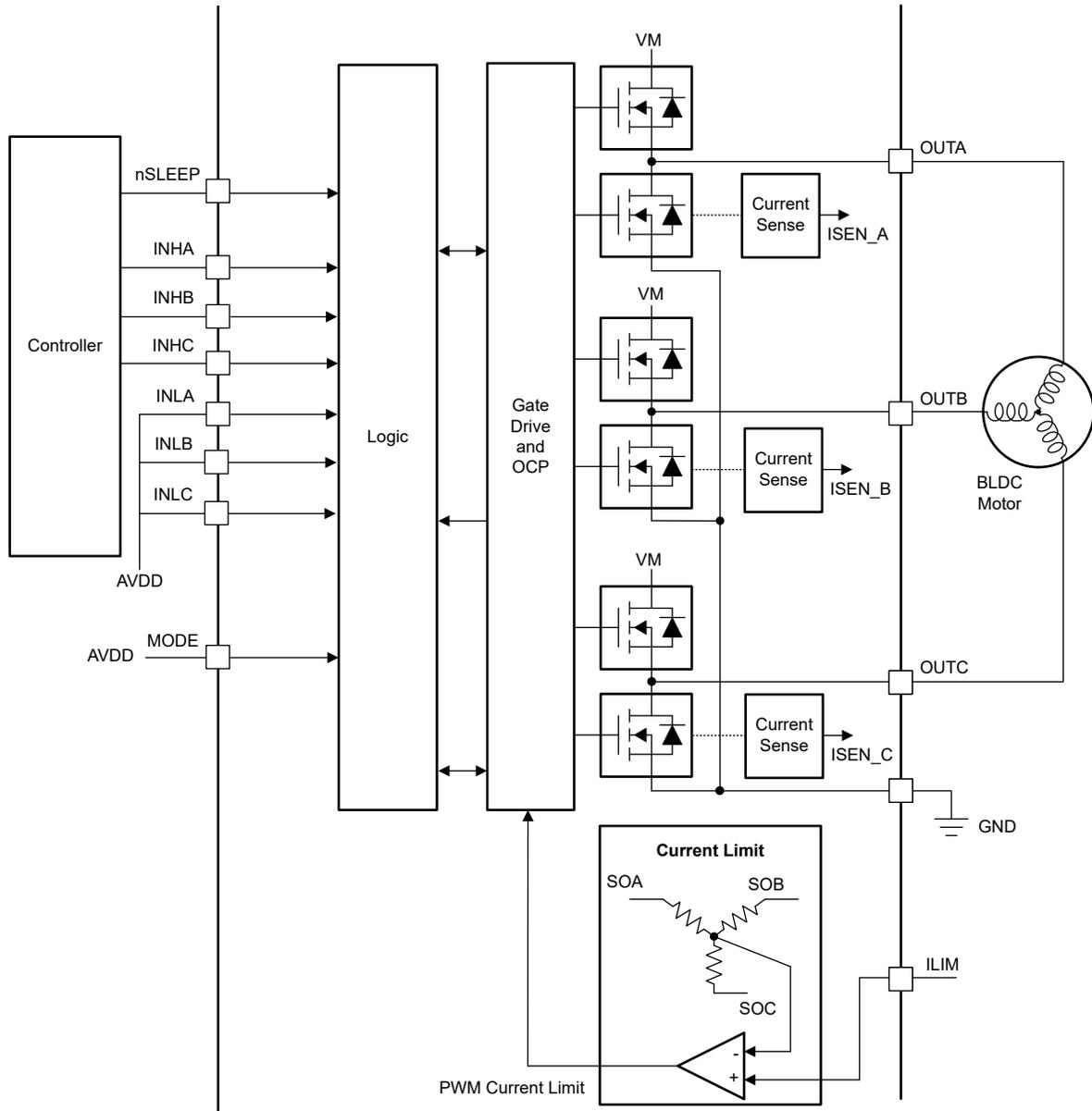
**Figure 8-6. 3x PWM Mode with Current Limit**
