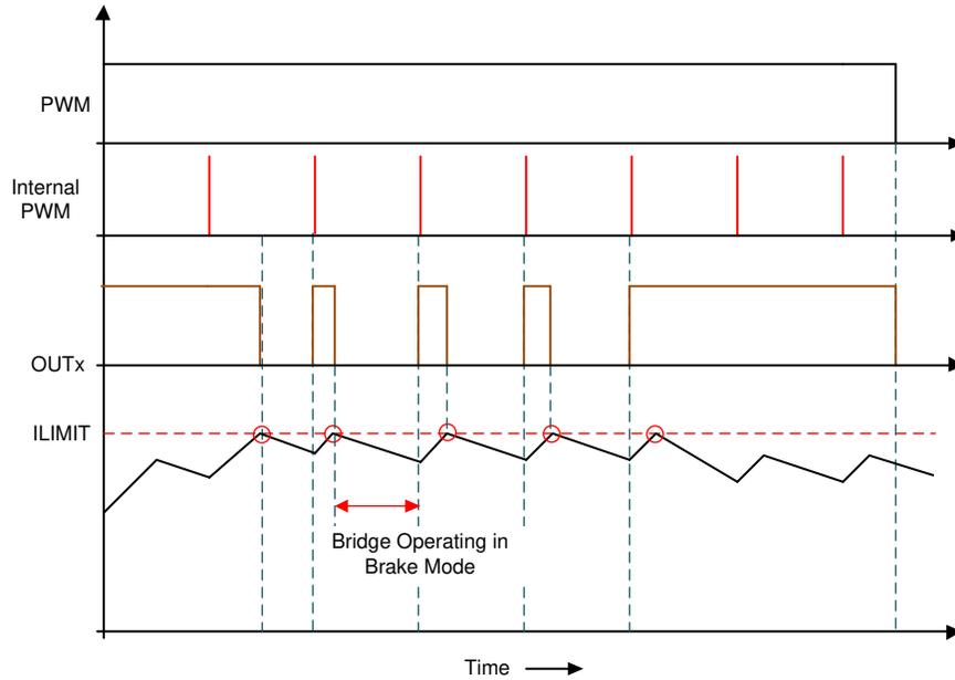
**Figure 8-40. Cycle-by-Cycle Current-Limit Operation with 100% PWM Duty Cycle**
