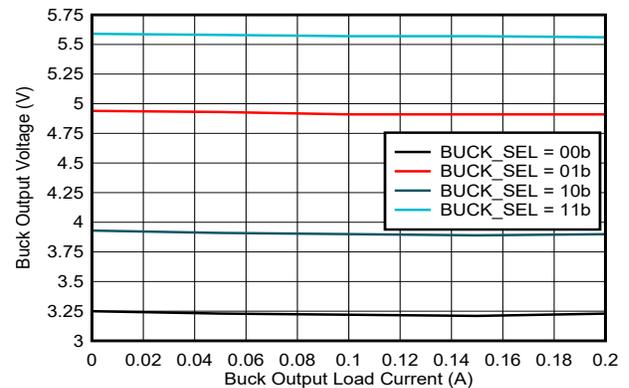
Figure 7-5. Buck regulator output voltage over load current
