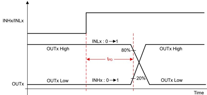
Figure 8-20. Propagation Delay
