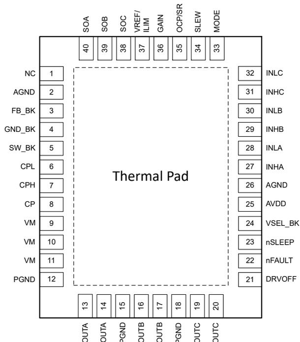
**Figure 6-2. DRV8316CT-Q1 40-Pin VQFN With Exposed Thermal Pad Top View**
