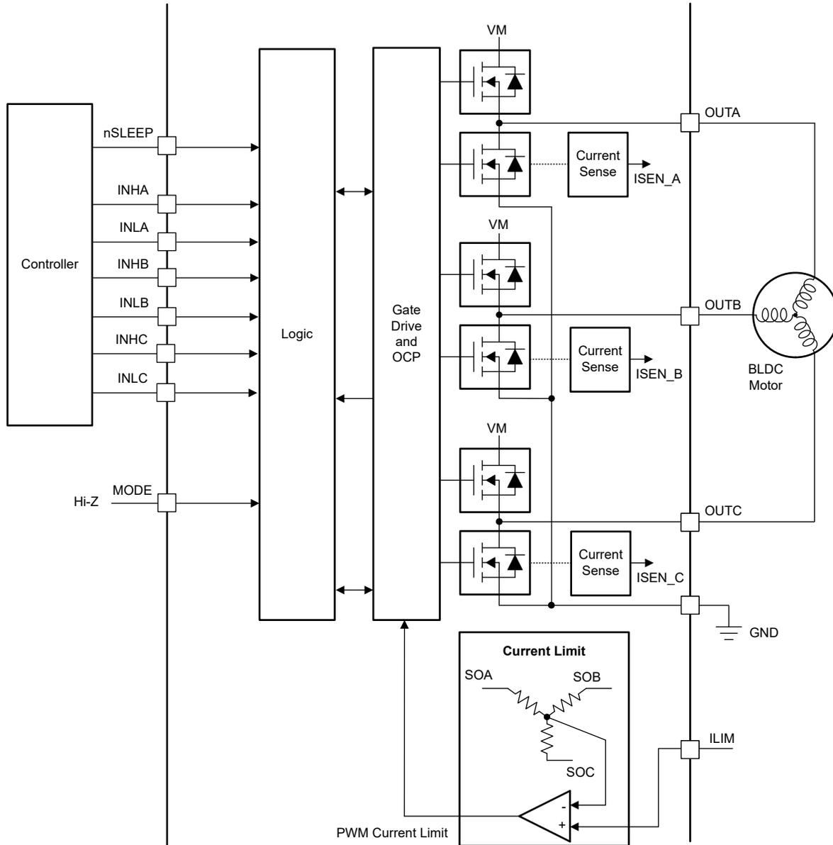
**Figure 8-5. 6x PWM Mode with Current Limit**
