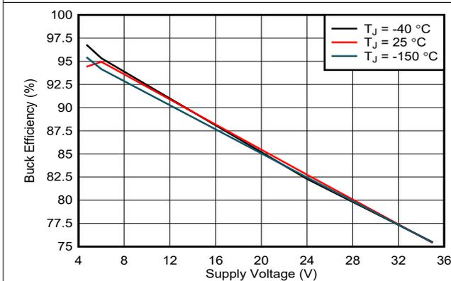
Figure 7-4. Buck regulator efficiency over supply voltage
