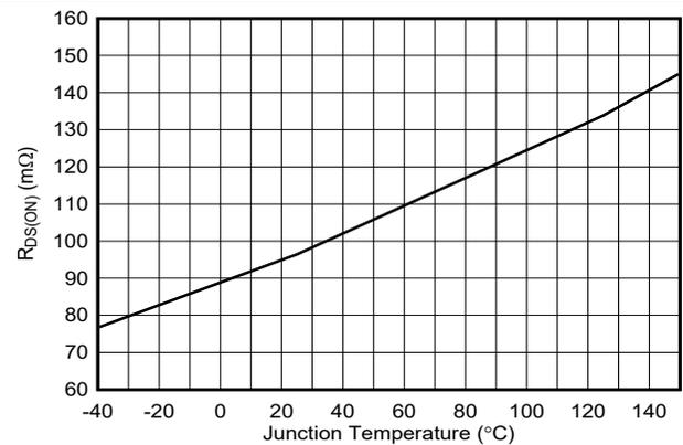
Figure 7-3. R<sub>DS(ON)</sub> (high and low side combined) for MOSFETs over temperature
