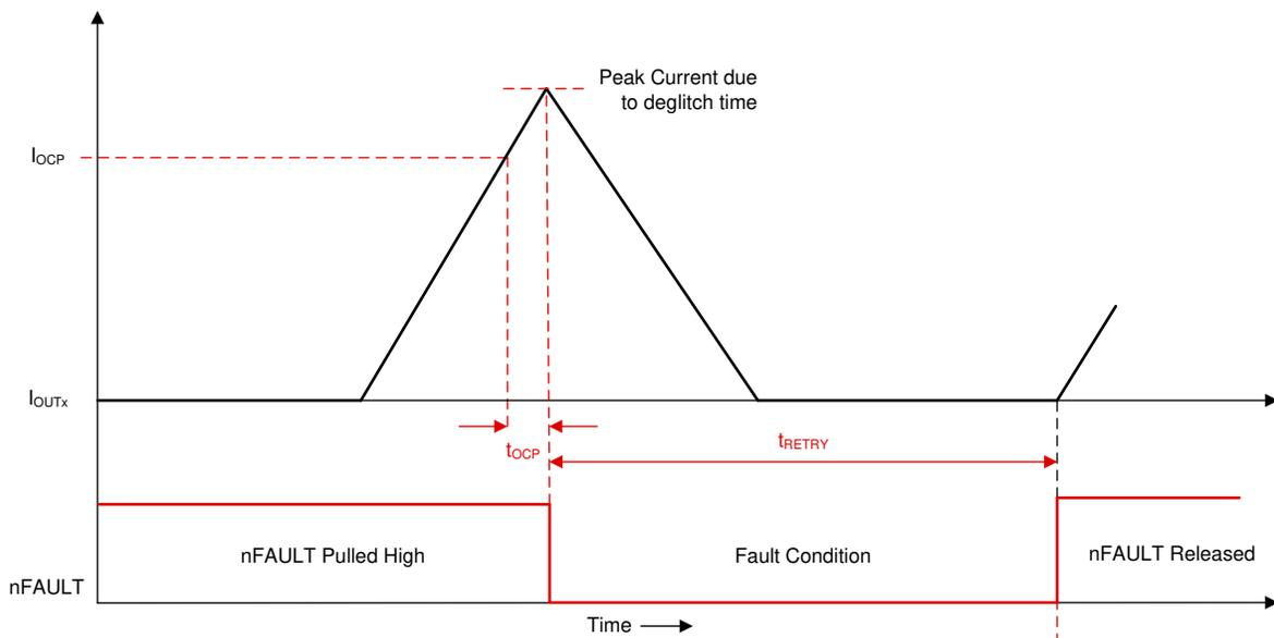
**Figure 8-44. Overcurrent Protection - Automatic Retry Mode**
