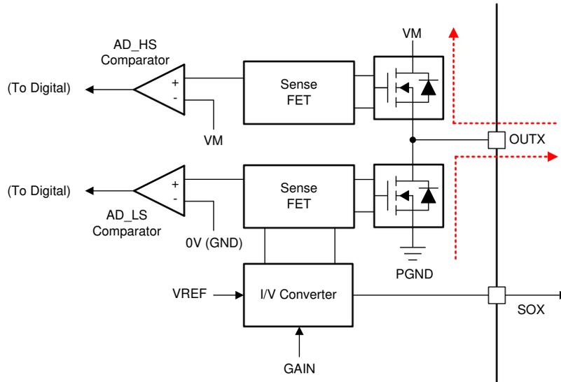
**Figure 8-31. Active Demagnetization Operation**
