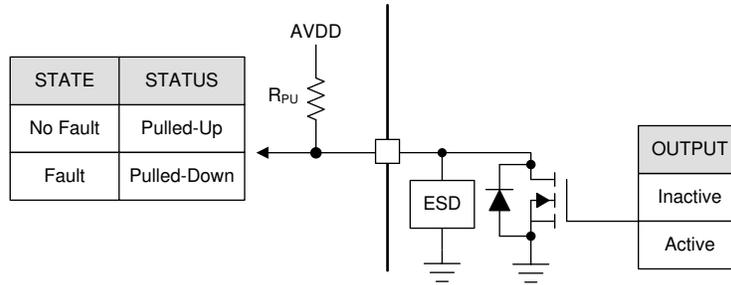
Figure 8-25. Open Drain
