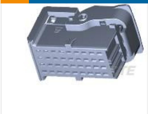
TE Part #1-1718485-1 CARRIER FOR RECEPT. INSERTS 36 POS
