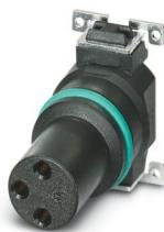
Contact carrier, 3-position, Socket, straight, M8, coding: A, PCB mounting, SMD reflow, Alternative product in accordance with RoHS II without Exemption 6c (Pb < 0.1 %) item no.: 1308271
