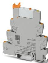
PLC-INTERFACE, consisting of PLC-BPT.../21 basic terminal block with Push-in connection and plug-in miniature relay with power contact and manual operation, 1 changeover contact, 120 V AC/110 V DC input voltage
