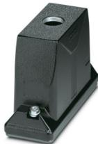
Sleeve housing B24, with screw locking, material: Die-cast aluminum, salt water resistant, cable outlets: 1, straight, 1x M25, height: 93.7 mm, cable gland: none, increased environmental requirements
