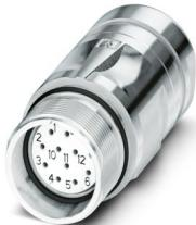
M23, Coupler connector, series: CA, straight, shielded: yes, for standard and SPEEDCON interlock, No. of pos.: 17, Direction of rotation: Standard, contact connection type: Socket, Solder connection, cable diameter range: 4 mm ... 6 mm, coding: N, Alternative product in accordance with RoHS II without Exemption 6c ( $Pb < 0.1\%$ ) item no.: 1244015
