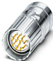
M23, Cable connector, series: CA, straight, shielded: yes, Screw locking mechanism, No. of pos.: 17, Direction of rotation: Standard, contact connection type: Pin, Solder connection, cable diameter range: 4 mm ... 6 mm, coding: N, Alternative product in accordance with RoHS II without Exemption 6c (Pb < 0.1 %) item no.: 1243781
