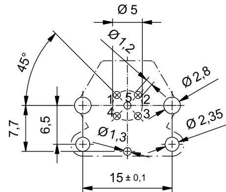
**Front panel section**
