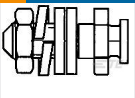
TE Part #5206514-1 SLIDING LOCK POST KIT
