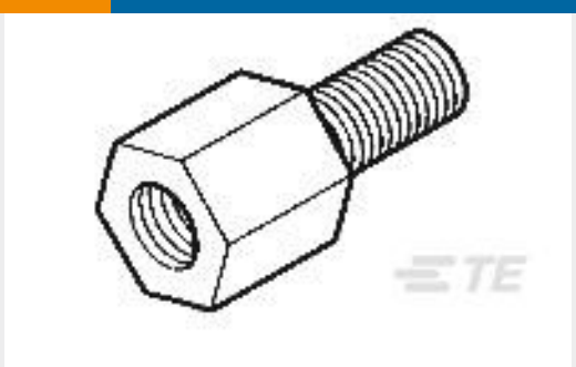
TE Part #1376059-1 FIXED HEAD SCREW FOR DYNAMIC
