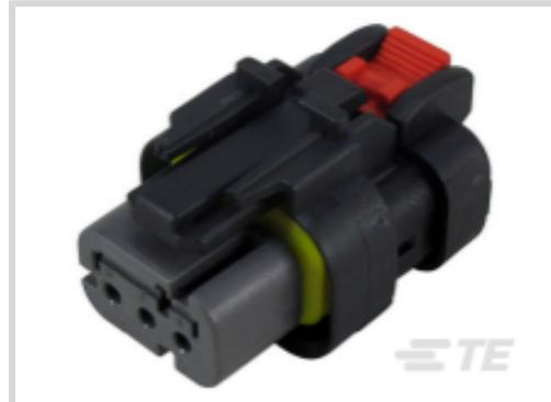
Connector System: **Wire-to-Wire**Number of Positions: **3**Connector & Housing Type: **Plug**Centerline (Pitch): **4.5 mm [.177 in]**Sealable: **Yes**[All AMPSEAL 16 Housings \(224\)](#)
