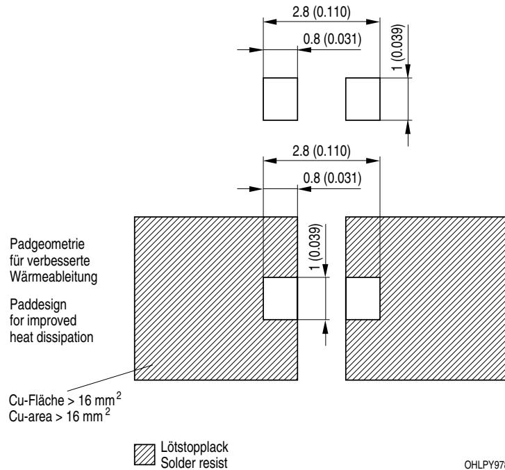
For superior solder joint connectivity results we recommend soldering under standard nitrogen atmosphere. Package not suitable for ultra sonic cleaning.
