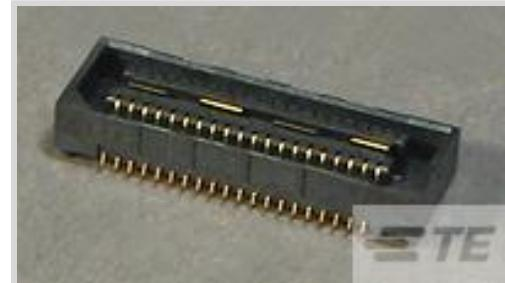
PCB Connector Assembly Type: **PCB Mount Receptacle**PCB Mount Orientation: **Vertical**Connector System: **Board-to-Board**Number of Positions: **28**Centerline (Pitch): **.8 mm [.031 in]**
