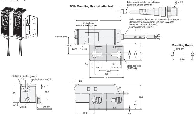
\*The Mounting Bracket can be attached to side A.
