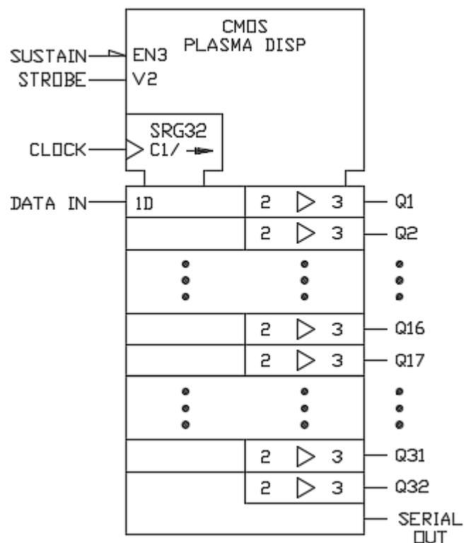
FIGURE 3. Logic symbols and functional block diagrams – continued.
