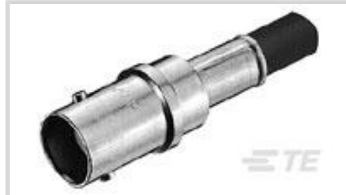
RF Interface: **BNC**RF Connector Style: **Jack**RF Connector Mated Outer Diameter (Approximate): **14.53 mm [ .572 in ]**Impedance: **50 Ω**Compatible With RF Cable Type: **RG 59, RG 59A, RG 59B, RG 62, RG 62A, RG 62B**
