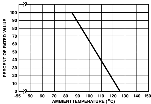
Figure 1A - Power Derating for Epoxy Coated
