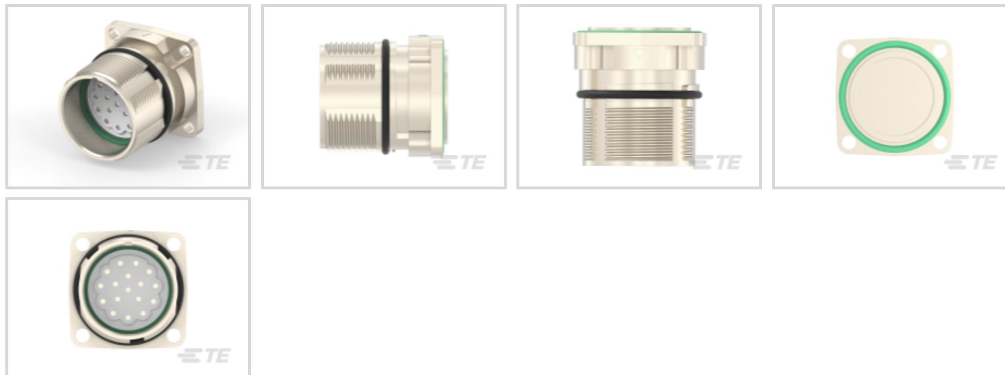
Connector System: **Cable-to-Panel**Connector Mounting Type: **Panel Mount**Sealable: **No**Circuit Application: **Signal**Shell Plating Material: **Electrodeposited Nickel**
