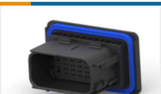
TE Part #2272889-4 24POS,AMPSEAL 16,PIN HSG ASSY, SLD,COD D
