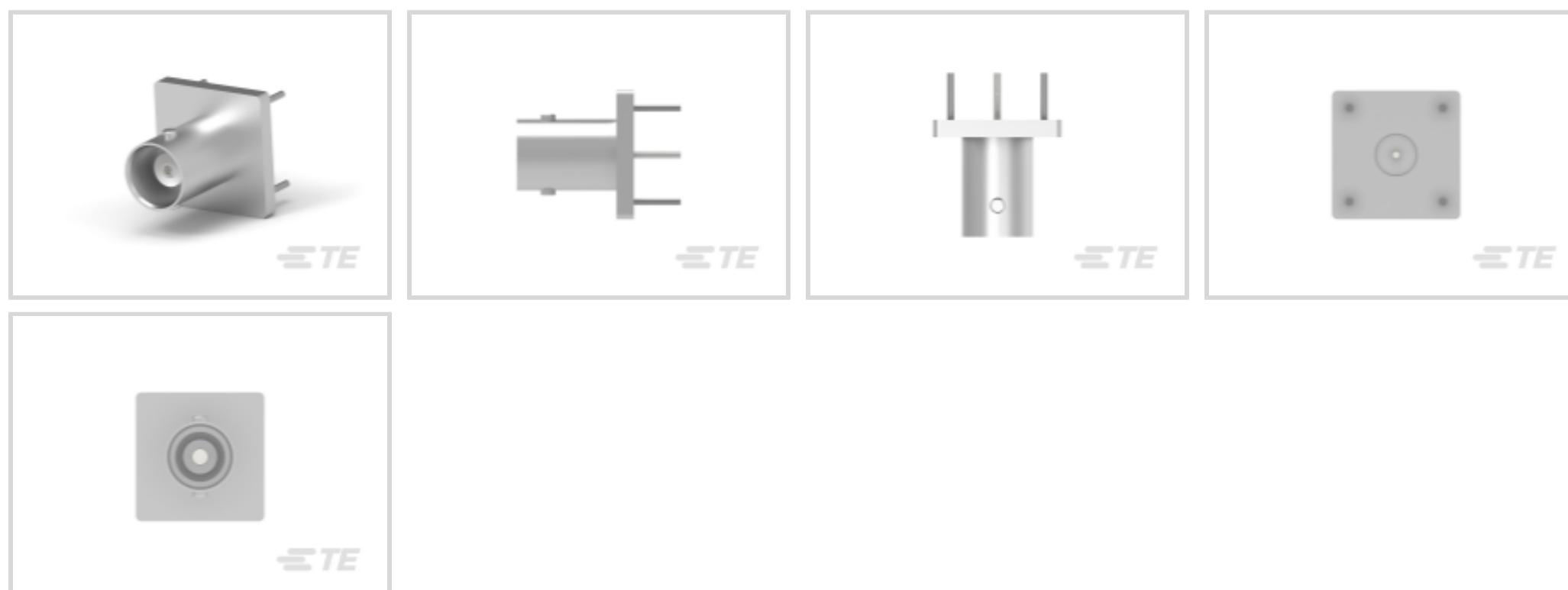
RF Interface: **BNC**RF Connector Style: **Jack**RF Connector Mated Outer Diameter (Approximate): **14.53 mm [ .572 in ]**Impedance: **50 Ω**RF Connector Coupling Mechanism: **Bayonet**[All BNC Vertical Jack RF Connector, 50 Ohm, Bayonet Coupling Mechanism \(28\)](#)
