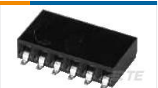
TE Part #1-969973-0 2x10P HV100 REC. CON, SMD, GOLD, BLISTER
