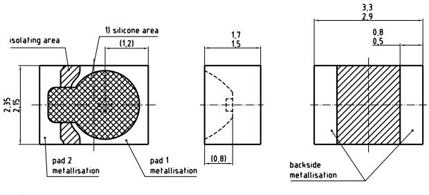
Device casted with silicone. Avoid mechanical stress on silicone surface.
