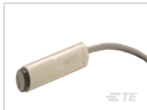
Humidity Sensor Product Type: **RH Module**Supply Voltage (Peak): **5.5 VDC**Operating Temperature Range: **-40 – 60 °C [ -40 – 140 °F ]**Accuracy: **±3 %RH**Current Consumption: **1.4 mA**
