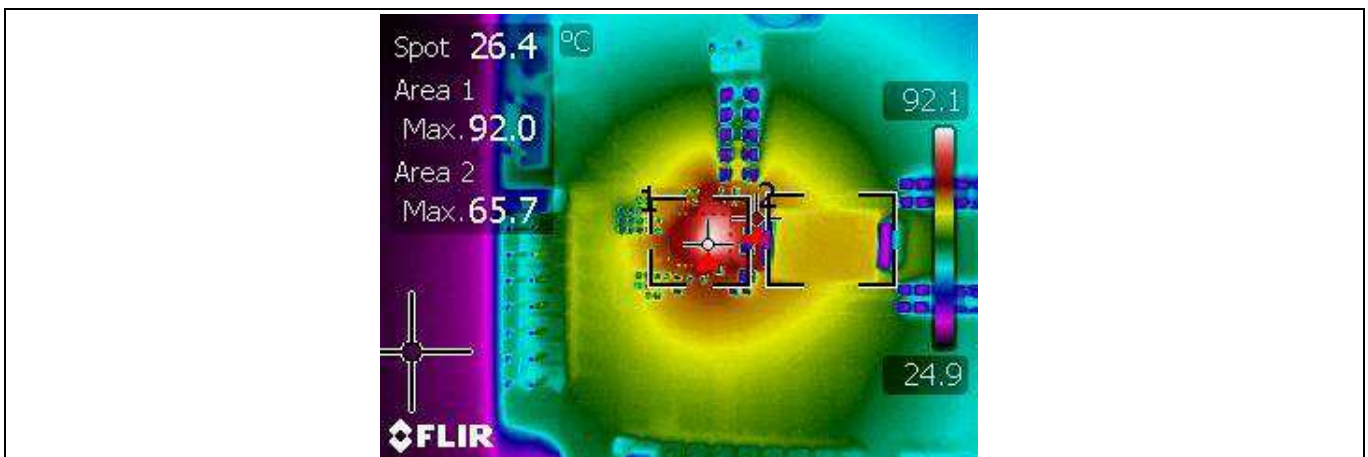
Figure 22 Thermal image of the board at 25 A load TDA38827 = 92°C, L = 65.7°C, fsw = 800 kHz, room temperature, natural convection
