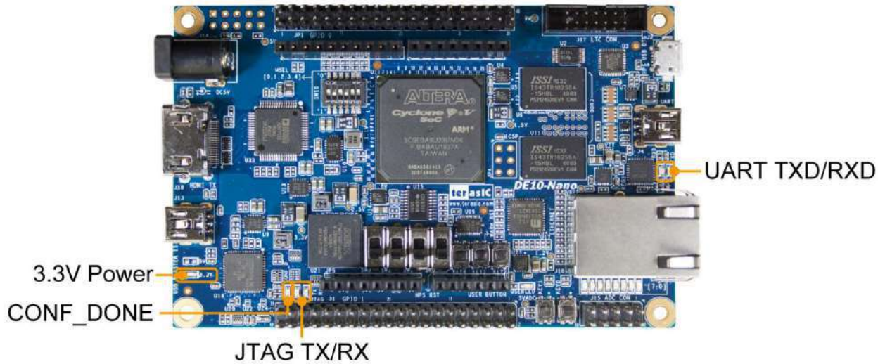
Figure 3-12 LED Indicators on DE10-Nano
