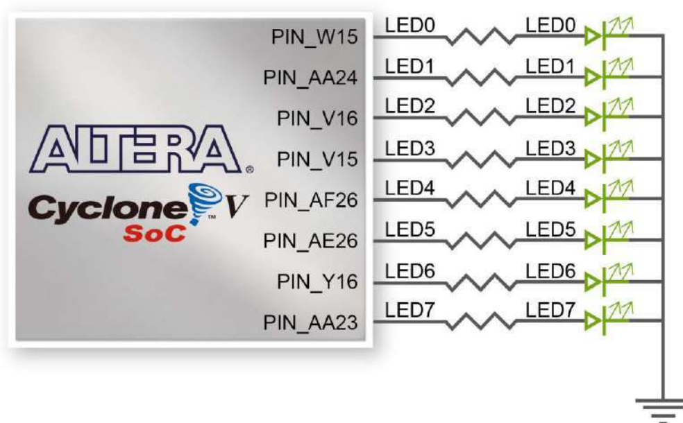
Figure 3-19 Connections between the LEDs and the Cyclone V SoC FPGA
