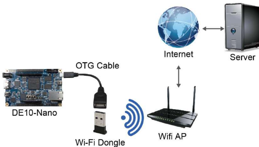
Figure 6-9 System diagram of USB Wi-Fi dongle
