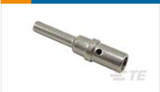
TE Part #0460-204-12141 PIN, SOLID, SIZE 12, 12-14AWG, NI
