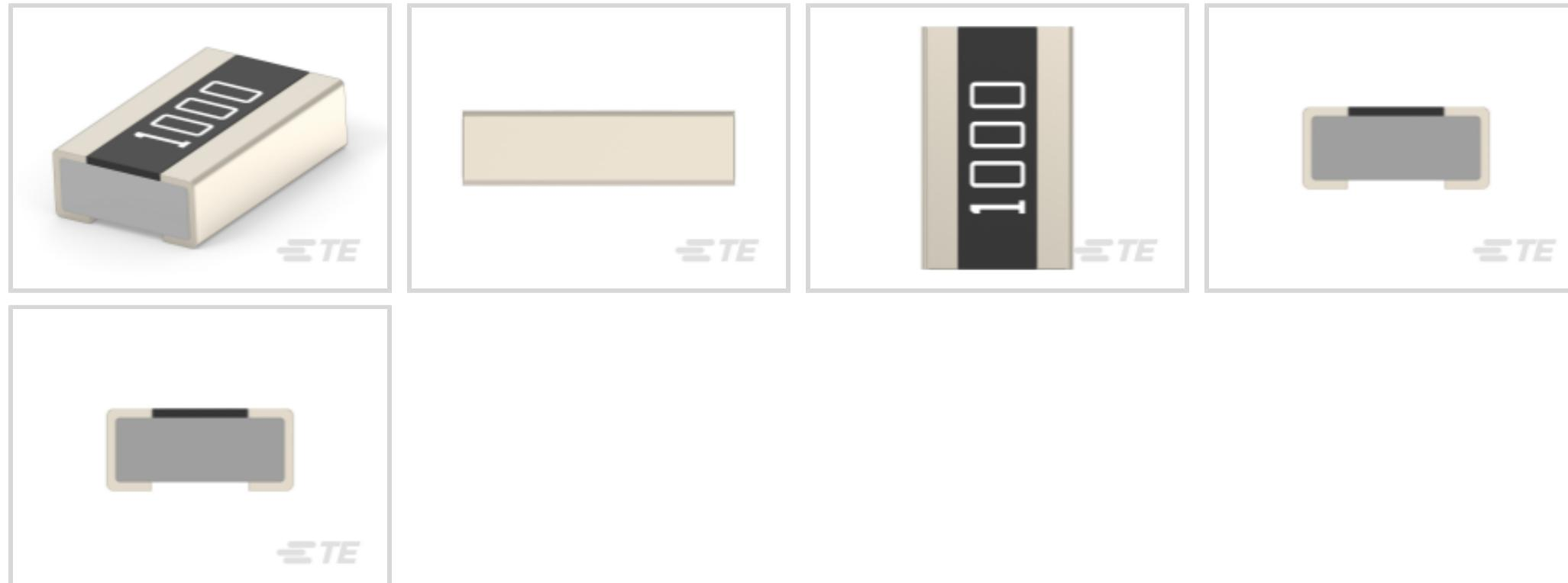
Resistor Type: **Power Resistor**Element Type: **Thick Film**Package Size Code: **0508**Power Rating: **1 W**Resistance Value: **680  $\Omega$**
