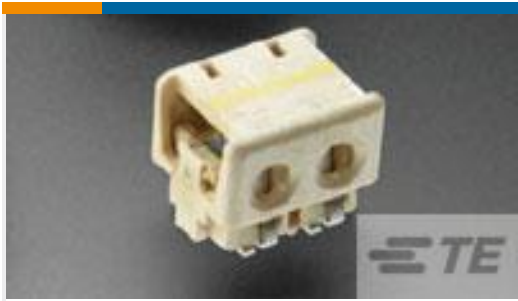
TE Part #2-2106003-3 Connector, SMT-IDC, 3 position, 22AWG
