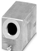
Sleeve housing B16, for single locking latch, material: Die-cast aluminum, salt water resistant, cable outlets: 1, lateral, 1x Pg21, height: 60 mm, cable gland: none, Standard
