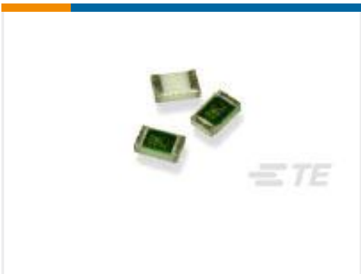
TE Part #5-1879215-4 CPF 0402 16K2 0.1% 25PPM 1K RL
