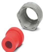
Half screw connection Pg16, made of plastic, consisting of rubber seal with one hole and one pressure screw, for type 1 housings, cable [mm] 9 - 13
