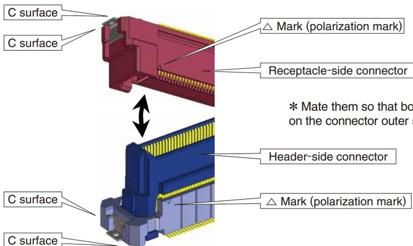
\* Mate them so that both C surfaces or both △ marks on the connector outer surface are aligned.
