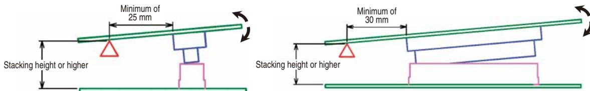
●This connector has a floating structure, but the floating range may vary depending on the height of connector on the header side (which has a floating mechanism).
