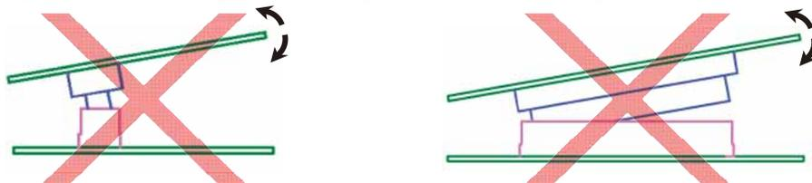
If you have no choice but to mate and un-mate with prying force based on your usage environment, use a point as a pivot shown by △ mark in the figure below when you apply those forces. The point shall be a certain distance away from the connector end and has equal or higher height of the mating height.
