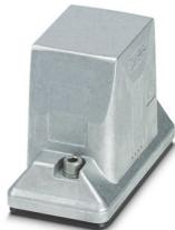
Sleeve housing B10, with screw locking, material: Die-cast aluminum, salt water resistant, variable, height: 74 mm, cable gland: none, Offshore/EMC, Without thread opening for screw connection, conductive seal (EMC properties)
