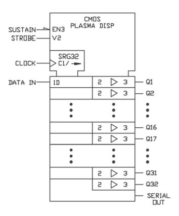
FIGURE 3. <u>Logic symbols and functional block diagrams</u> – continued.
