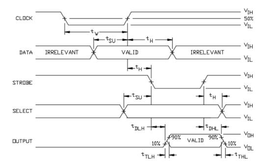
FIGURE 4. Switching waveforms.
