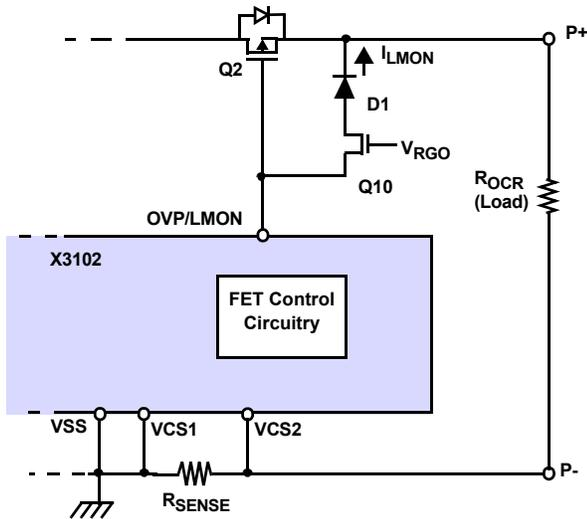
FIGURE 13. OVERCURRENT PROTECTION
