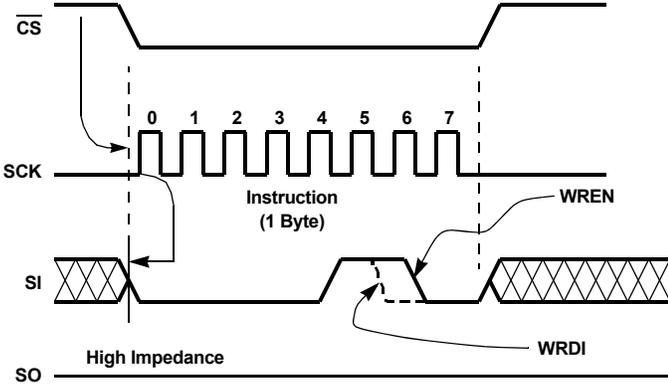
**FIGURE 17. EEPROM WRITE ENABLE LATCH (WREN/WRDI) OPERATION SEQUENCE**
