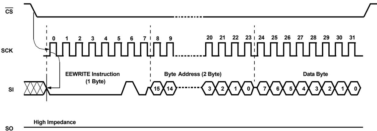
**FIGURE 18. EEPROM BYTE WRITE (EWRITE) OPERATION SEQUENCE**
