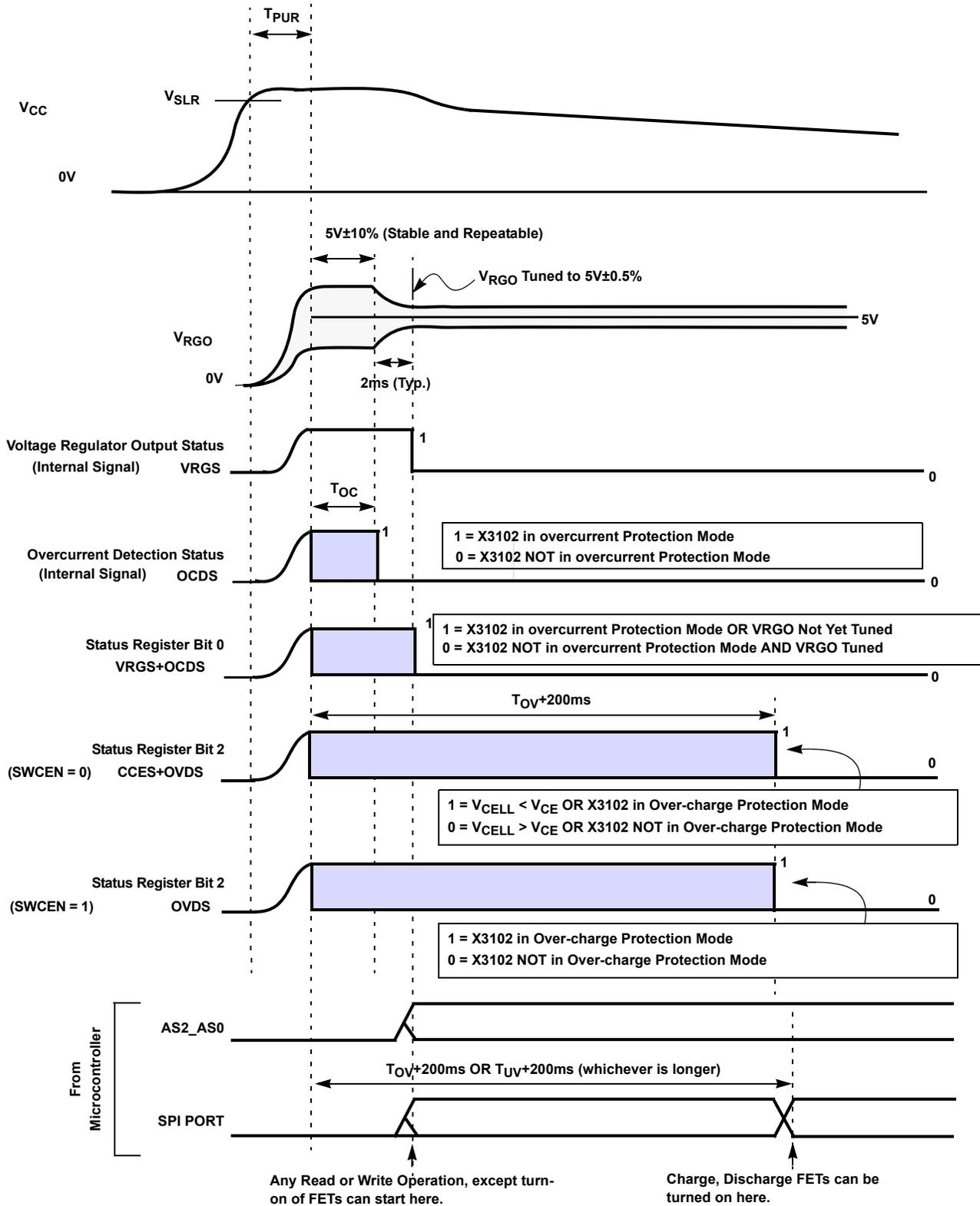
FIGURE 8. POWER UP TIMING (INITIAL POWER UP OR AFTER SLEEP MODE)
