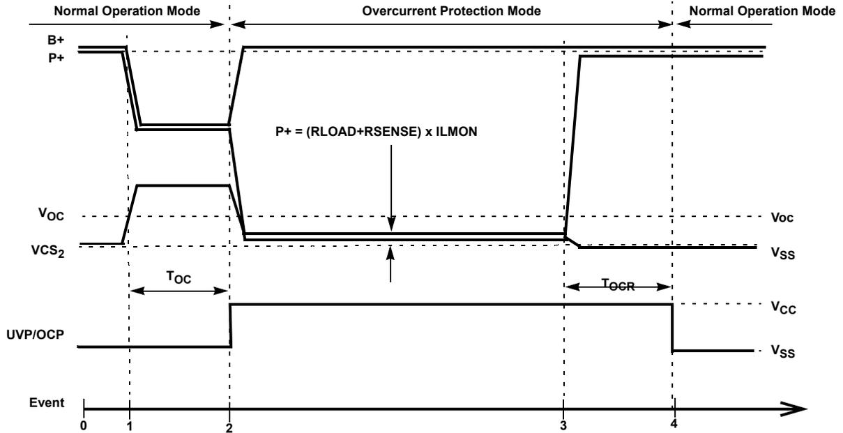
FIGURE 14. OVERCURRENT PROTECTION MODE - EVENT DIAGRAM
