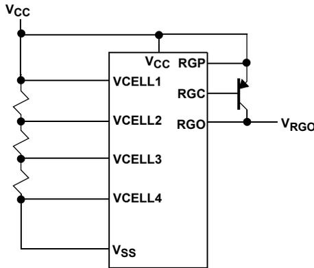
Increase V<sub>cc</sub> until V<sub>RGO</sub> turns on
