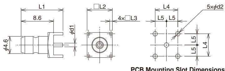
PCB Mounting Slot Dimensions
