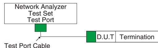
Note 1 : The cable connector is measured with the connector attached to the applicable cable at 10cm from both ends.
