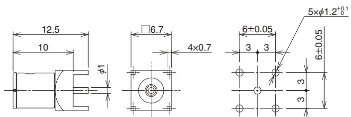
PCB Mounting Slot Dimensions
