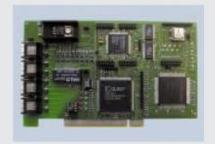
The MUNICH128X is compatible with the LAPD ISDN (Integrated Services Digital Network) protocol specified by CCITT, as well as with HDLC, SDLC, LAPB and DMI protocols. It provides rate adaption for time-slot transmission from 64 kbit/s down to 8 kbit/s and the concatenation of time-slots, supporting the ISDN H0, H11, H12 superchannels.
