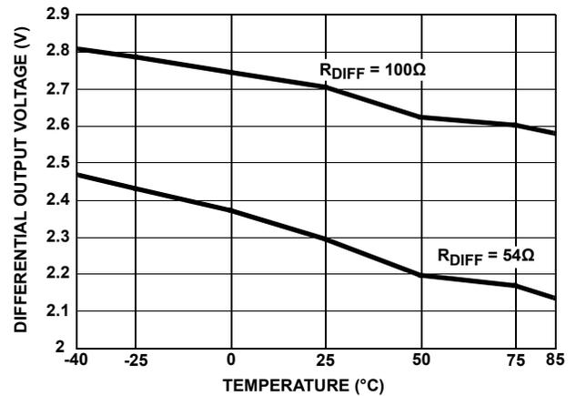
FIGURE 10. DRIVER DIFFERENTIAL OUTPUT VOLTAGE vs TEMPERATURE
