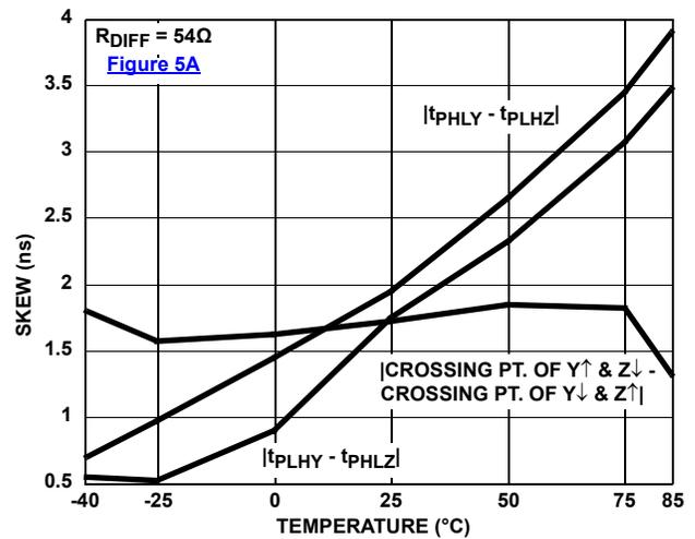
FIGURE 16. DRIVER SKEW vs TEMPERATURE (ISL83485, ISL83490, ISL83491)
