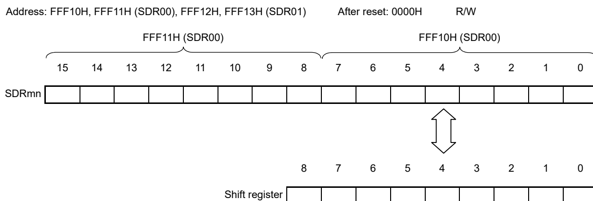
Figure 19 - 2 Format of Serial data register mn (SDRmn) (mn = 00, 01)
