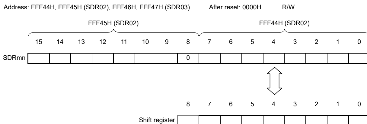
Figure 19 - 3 Format of Serial data register mn (SDRmn) (mn = 02, 03)
