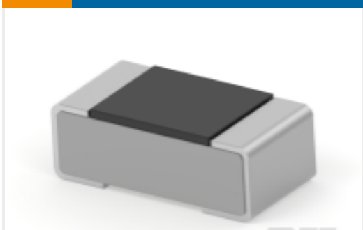
TE Part #2-2176338-1 CRGCQ 0402 2K2 5%
