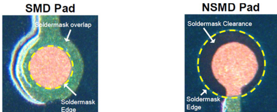
Figure 28. Solder mask (SMD) and non-solder mask defined (NSMD) pads
