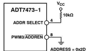
Figure 15. SMBus Address = 0x2D (Pin 4 = 1)
