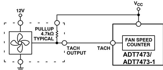
**Figure 40. Fan with TACH Pullup to V<sub>CC</sub>**
