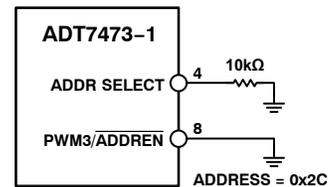
Figure 14. SMBus Address = 0x2C (Pin4 = 0)
