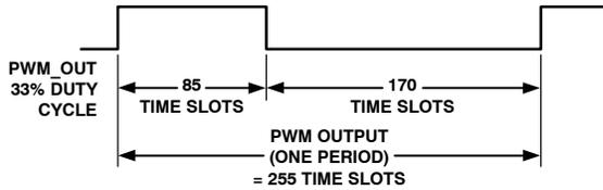
**Figure 75. 33% PWM Duty Cycle Represented in Time Slots**
