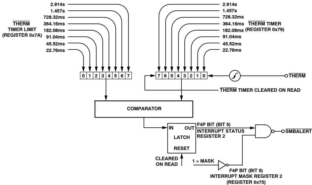
Figure 33. Functional Block Diagram of the ADT7473 THERM Monitoring Circuitry
