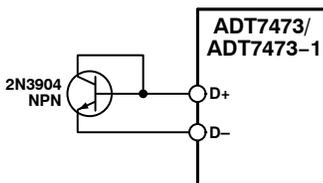
**Figure 25. Measuring Temperature Using an NPN Transistor**
