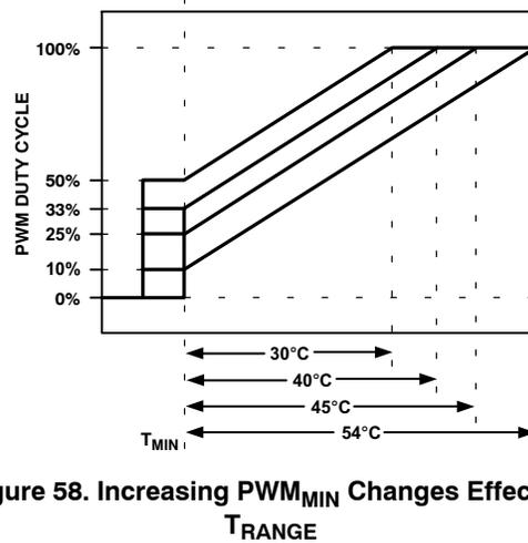
**Figure 58. Increasing PWM<sub>MIN</sub> Changes Effective T<sub>RANGE</sub>**
