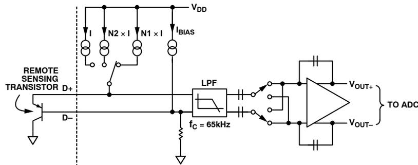
**Figure 24. Signal Conditioning for Remote Diode Temperature Sensors**
