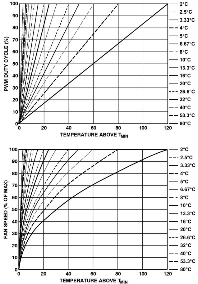
**Figure 59.  $T_{RANGE}$  vs. Actual Fan Speed Profile**
