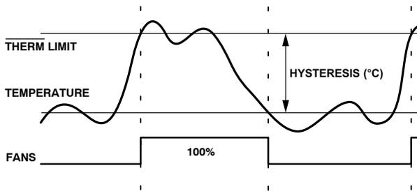
Figure 28. **THERM** Limit Operation
