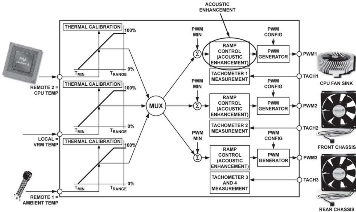
**Figure 74. Acoustic Enhancement Smooths Fan Speed Variations Under Automatic Fan Speed Control**
