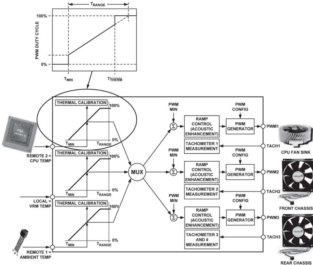
Figure 62. How  $\overline{THERM}$  Relates to Automatic Fan Control
