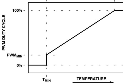
Figure 53.  $PWM_{MIN}$  Determines Minimum PWM Duty Cycle
