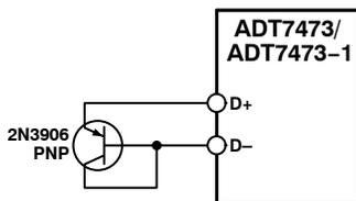
**Figure 26. Measuring Temperature Using a PNP Transistor**
