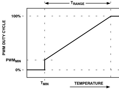
**Figure 56. T<sub>RANGE</sub> Parameter Affects Cooling Slope**
