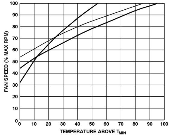
Figure 60.  $T_{RANGE}$  and % Fan Speed Slopes with  $PWM_{MIN} = 20\%$
