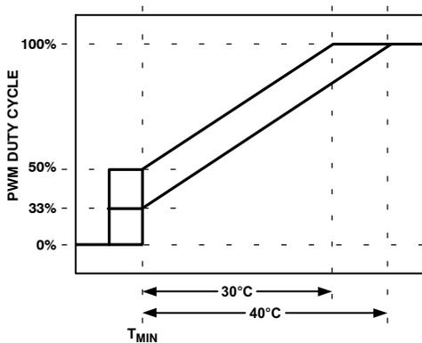
**Figure 57. Adjusting PWM<sub>MIN</sub> Affects T<sub>RANGE</sub>**
