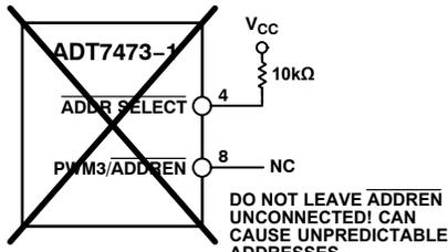
CARE SHOULD BE TAKEN TO ENSURE THAT PIN 8 (PWM3/ADDREN) IS EITHER TIED HIGH OR LOW. LEAVING PIN 8 FLOATING COULD CAUSE THE ADT7473-1 TO POWER UP WITH AN UNEXPECTED ADDRESS.
