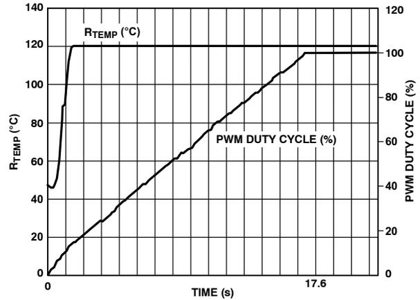
Figure 79. Enhanced Acoustics Mode with Ramp Rate = 2
