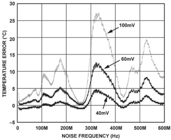
Figure 5. Remote Temperature Error vs. Common-Mode Noise Frequency
