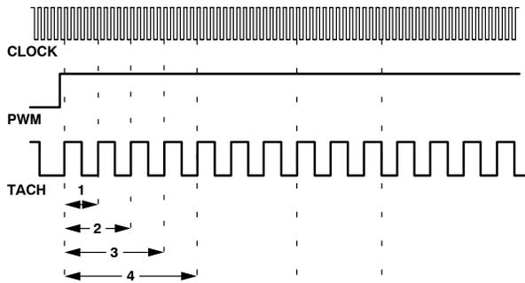
**Figure 44. Fan Speed Measurement**
